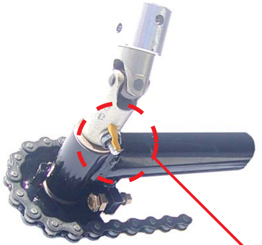
TAPER PIN INSTALLED VIEW A
