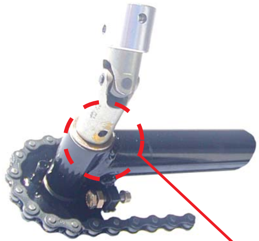
TAPER PIN REMOVED VIEW B
